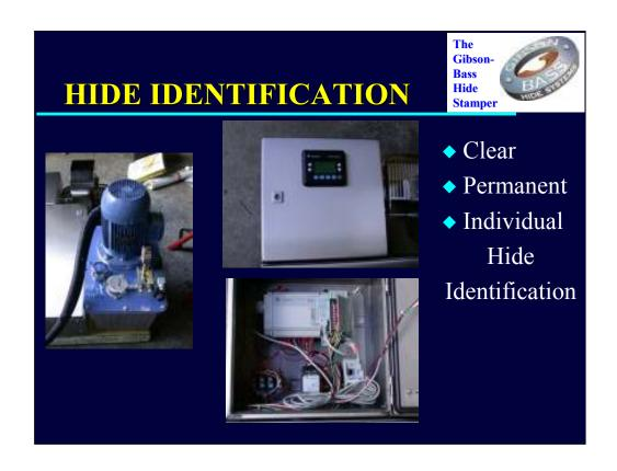
You can see the hydraulic pump, with a very powerful motor to drive the cutters right through. There is also the control box, which contains the HMI. Inside is the PLC, we use only Allen Bradley gear, which controls the stamping. It can communicate with you local computer system by ethernet or wireless.
